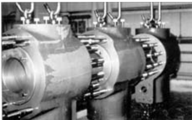
Figure 26 Electroless nickel plated mud pump bodies.
