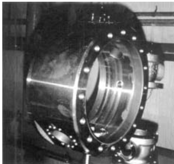
Figure 23 Electroless nickel plated body for large ball valve.
