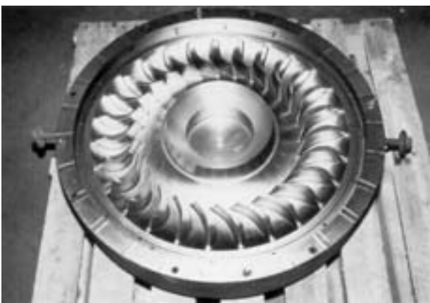
Figure 41 Electroless nickel is frequently used to protect foundry tooling such as this turbine core box.
