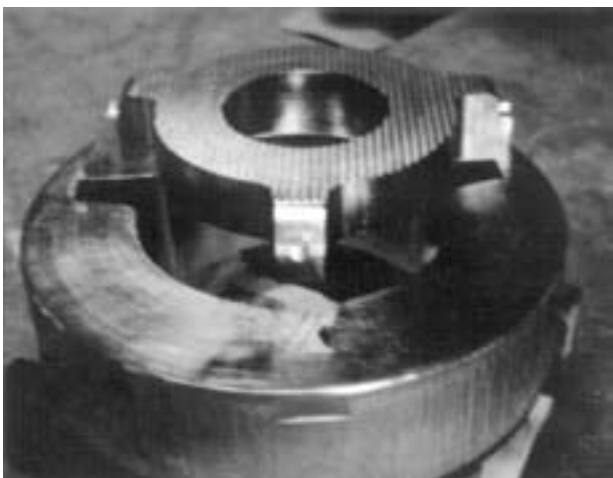
Figure 42 Wear resistance of electroless nickel has greatly improved productivity of molds for ceramic parts.
