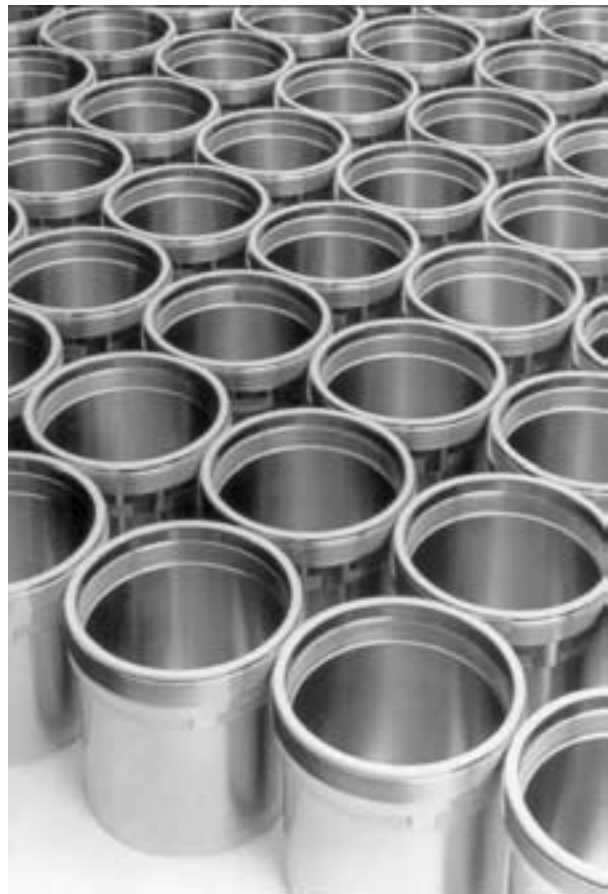
Figure 35 Steel missile directional canisters are plated with electroless nickel for corrosion protection.
