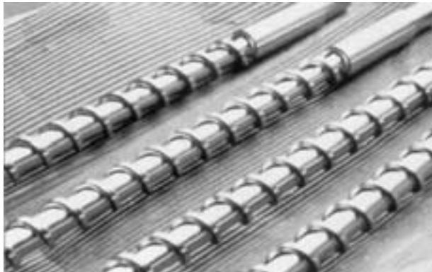
Figure 27 Corrosion and wear of down hole drill motor rotors are resolved by electroless nickel plus chromium plating.
