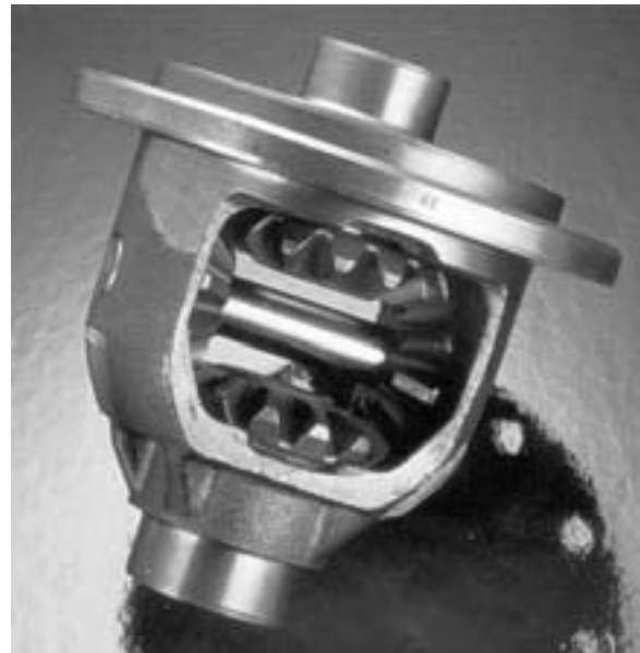
Figure 29 Plated pinion shafts in this differential have excellent wear and anti-galling properties.
